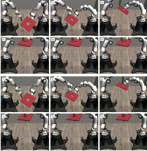
Figure 13. Full-rollout comparison on RoboSuite TWO-ARM PEG-IN-HOLE. The combined contact sheet contrasts a BRACE rollout that stabilizes replanning and successfully completes the task against the corresponding No-BRACE baseline, which repeatedly triggers replanning without controller-level budgeting or stabilization and ultimately fails.
